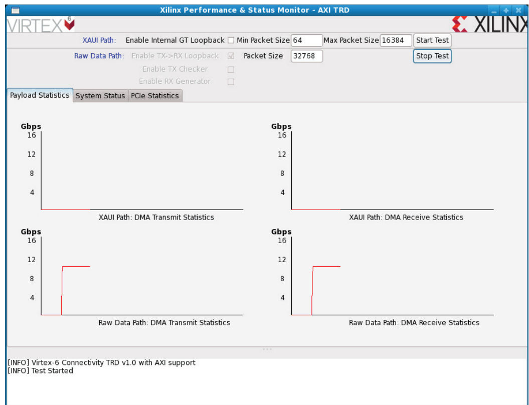
Figure 2-14: Test Setup and Payload Statistics Screen - Raw Data TX -> RX Loopback
