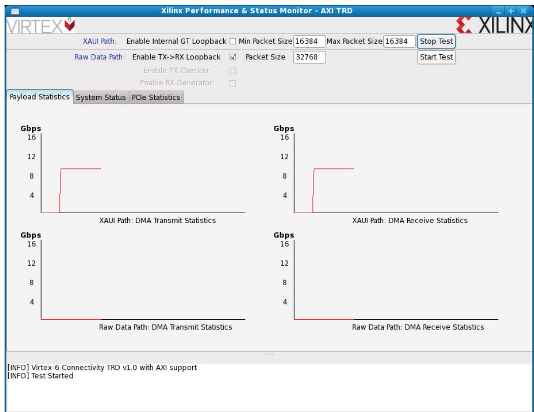
Figure 2-13: Test Setup and Payload Statistics Screen - XAUI Loopback
