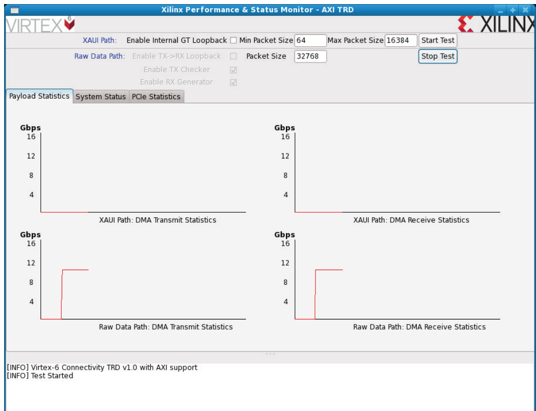
Figure 2-17: Test Setup and Payload Statistics Screen - Raw Data TX and RX
