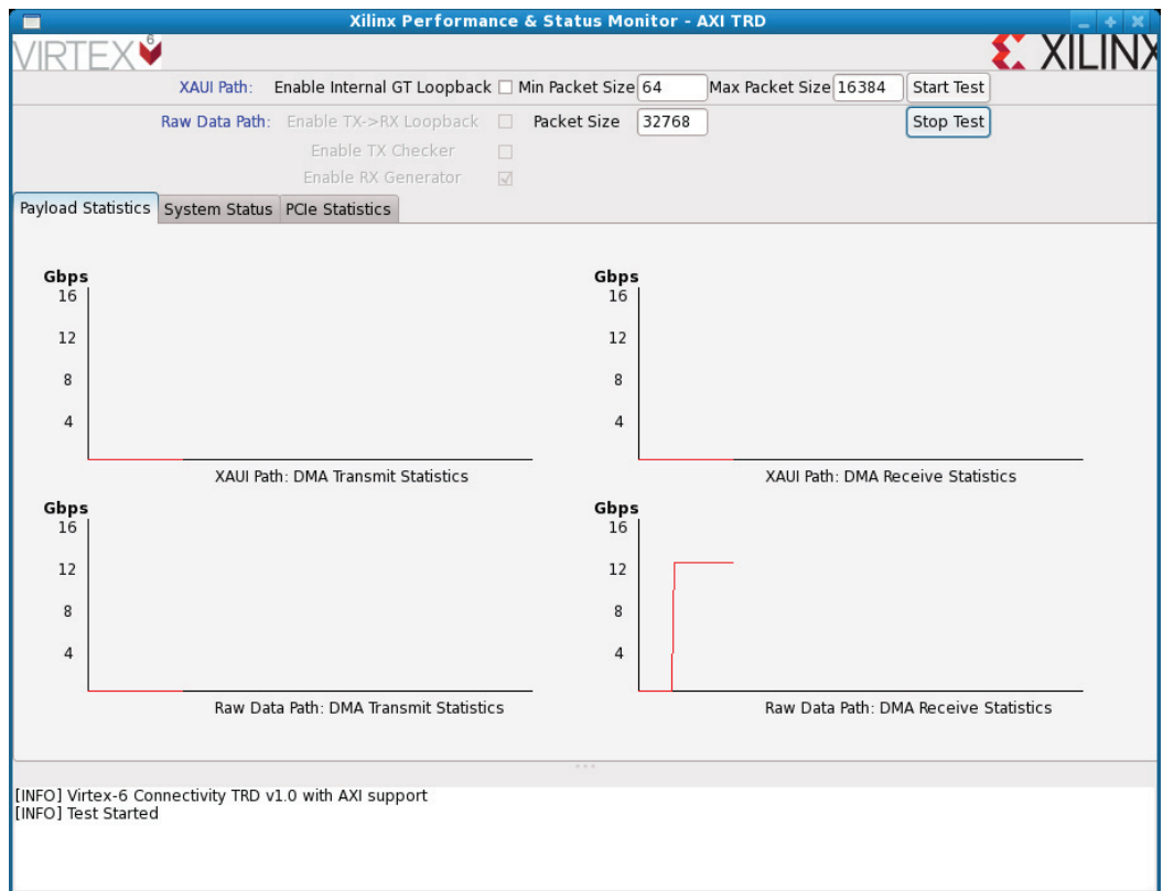
Figure 2-16: Test Setup and Payload Statistics Screen - Raw Data RX Only
