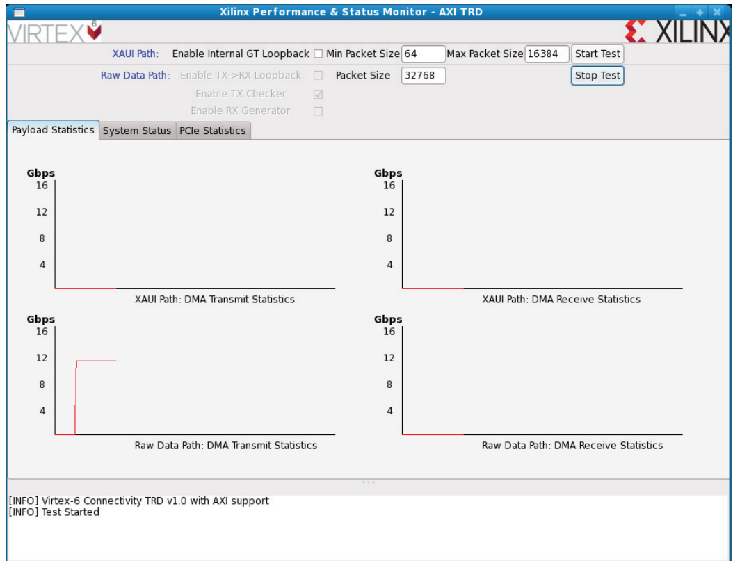
Figure 2-15: Test Setup and Payload Statistics Screen - Raw Data TX Only
