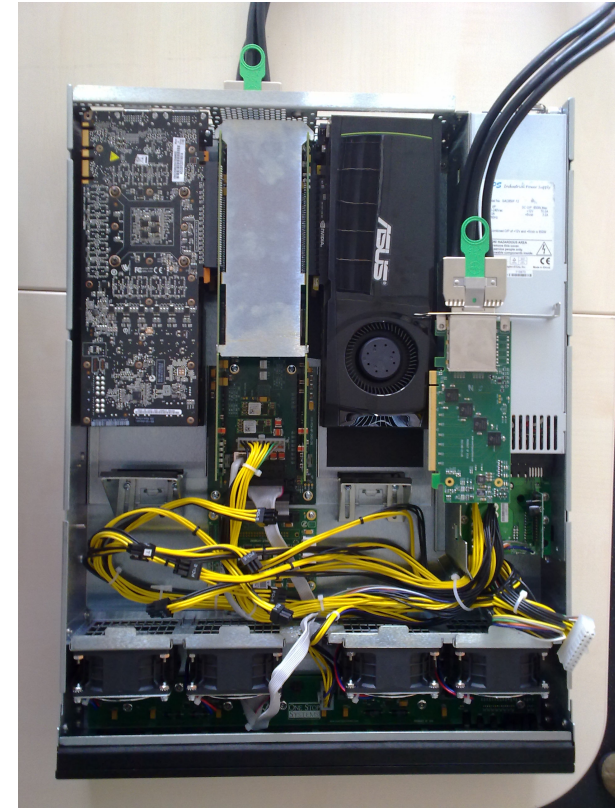
External GPU Box PCIe Interface Card (16x) 4 External GPUs 4600 EUR
