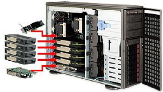
Imaging station equipped with 2 Xeon CPUs with in total 16 cores and 4 GPUs.
