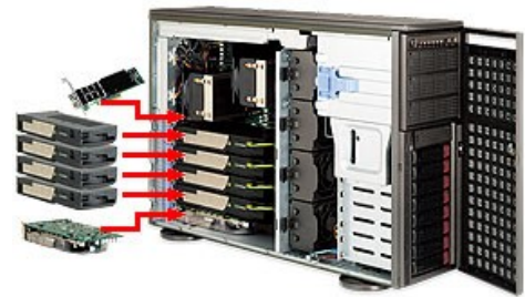
Imaging station equipped with 2 Xeon CPUs totaling to 16 computational cores and 4 GPUs.
