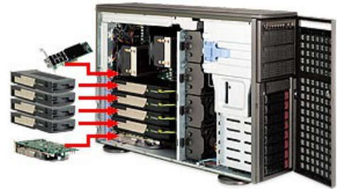
Imaging station equipped with 2 Xeon CPUs totaling to 16 computational cores and 4 GPUs.
